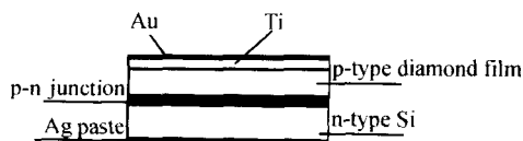
Fig. 1 Schematic diagram of the heterojunction between B doped diamond film and Si substrate
