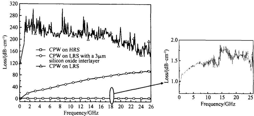
Fig. 4 Loss of the CPWs on HRS ,LRS , and LRS with a 3 $\mu$ m interlayer
