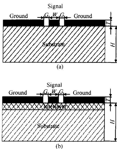
Fig. 1 (a) Cross section geometries of the standard CPW; (b) Cross section geometries of the CPW with an interlayer
