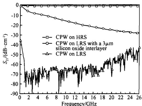
Fig. 2  $S_{21}$  of the CPWs on HRS, LRS, and LRS with a 3  $\mu\text{m}$  interlayer
