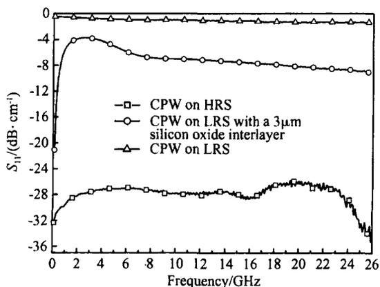
Fig. 3  $S_{11}$  of the CPWs on HRS, LRS, and LRS with a 3  $\mu\text{m}$  interlayer
