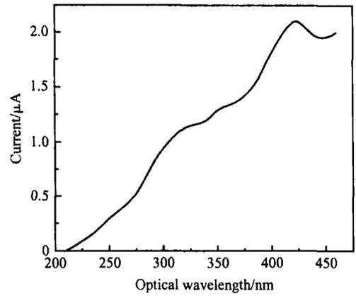
Fig. 6 Photo-current response at optical wavelengths
