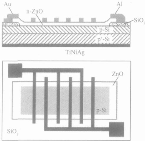
Fig. 1 Structure of the SHBT
