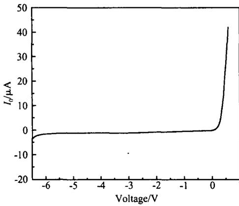
Fig. 5 I-V characteristics of n-ZnO/p-Si
