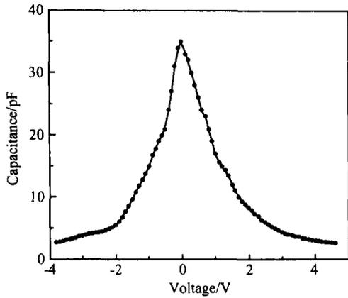
Fig. 4 C-V characteristics of Au/n-ZnO SBD
