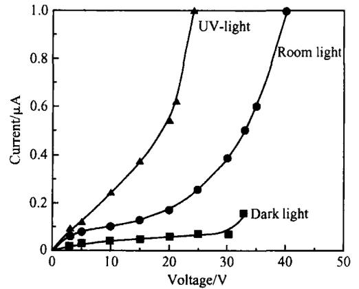
Fig. 3  $I$ - $V$  characteristics of Au/n-ZnO SBD
