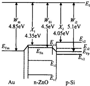
Fig. 2 Energy band of Au/n-ZnO/p-Si structure
