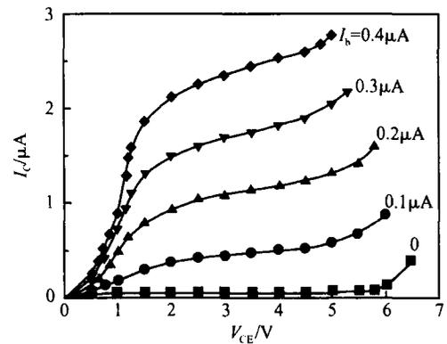
Fig. 7 UV light photocurrent response of SHBT for different VCE
