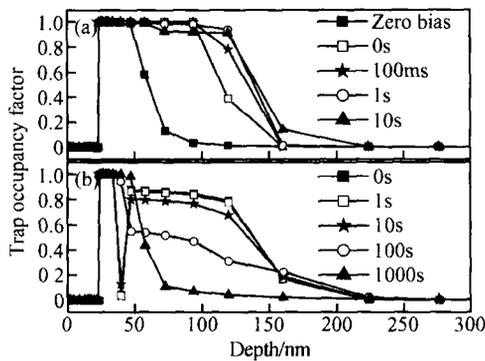
Fig.11 Change of the trap occupancy factor  $F_n$  with time at drain edge of the gate in the stress (a) and in the slow transient (b)
