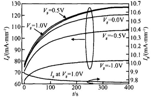
Fig. 6 Simulated transient curves at different  $V_g$
