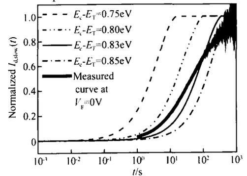
Fig. 4 Simulated  $I_{d,slow}(t)$  waveforms at different trap energy levels
