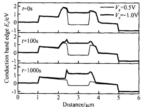
Fig. 7 Surface conduction band edge at different times for  $V_g = 0.5V$  and  $V_g = -1.0V$
