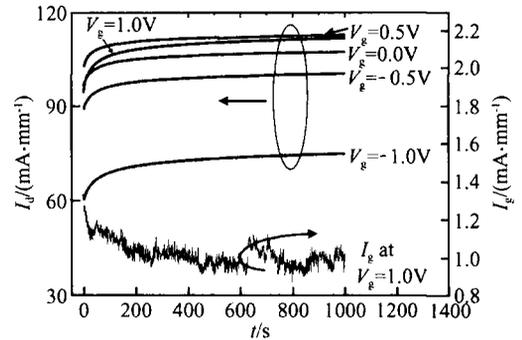
Fig. 2 Measured drain current transients at  $V_d = 1\text{V}$  under different  $V_g$ . The gate current at  $V_g = 1\text{V}$  is also shown.
