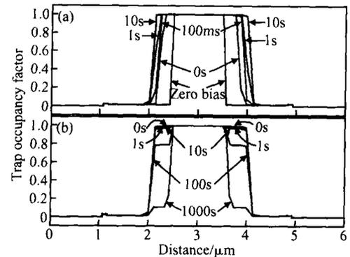
Fig. 9 Change of the trap occupancy factor  $F_n$  with time at 5nm below the surface in the stress (a) and in the slow transient (b)
