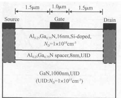
Fig. 1 Device structure The gray regions are taken to be GaN in the simulation.
