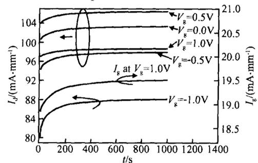
Fig. 10 Simulated transient curves at different  $V_g$
