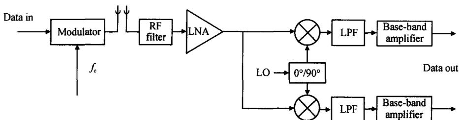
Fig. 2 Simplified zero IF transceiver architecture
