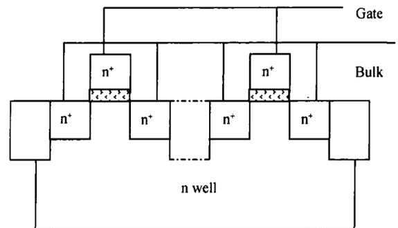
Fig. 8 Cross-section of a MOS varactor
