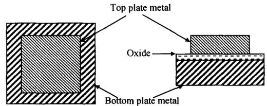
Fig. 10 MIM capacitor layout and cross-section
