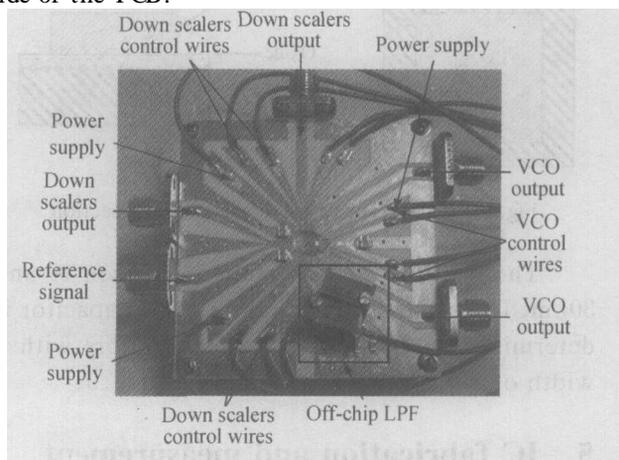
Fig. 12 Photograph of the test PCB
