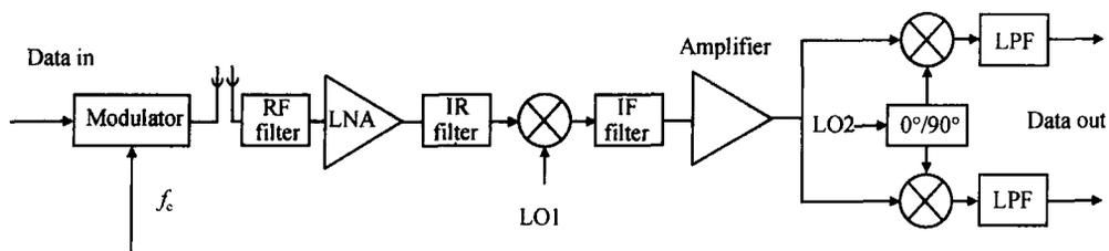
Fig. 1 Simplified heterodyne transceiver architecture
