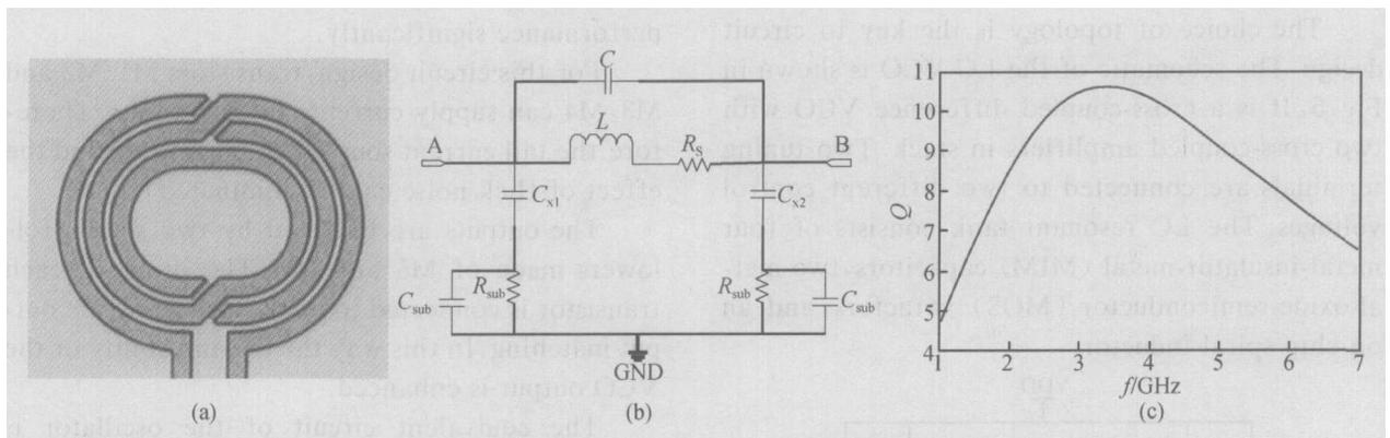
Fig. 7 (a) Microphotograph of the on-chip spiral inductor; (b) Model of the inductor; (c)  $Q$ -curve of the inductor
