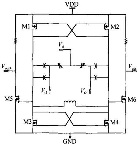
Fig. 5 Circuit schematic of the VCO
