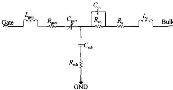
Fig. 9 Equivalent circuit of a MOS varactor
