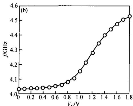
Fig. 13 Measured tuning characteristics of the VCO (a)  $V_{t1} = 0.8V$ ; (b)  $V_{t1} = 1V$
