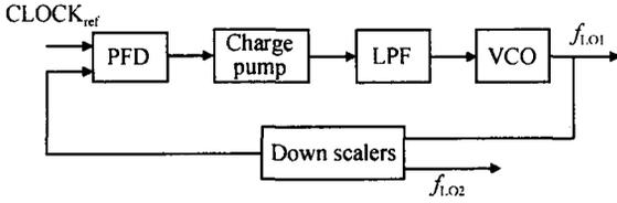
Fig. 4 Block diagram of the frequency synthesizer
