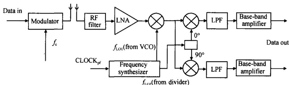
Fig. 3 Simplified dual frequency conversion transceiver architecture
