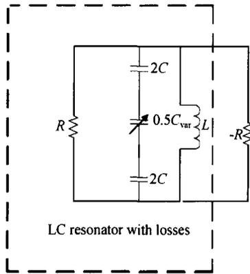
Fig. 6 Equivalent circuit of the oscillator
