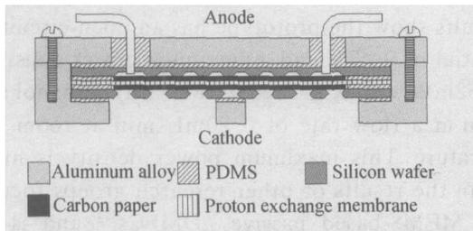
Fig. 1 Schematic of the air-breathing μDMFC
