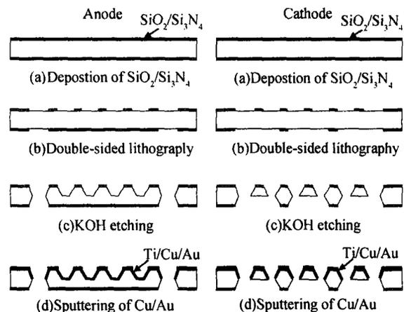
Fig. 4 Fabrication process of the anode and cathode plates
