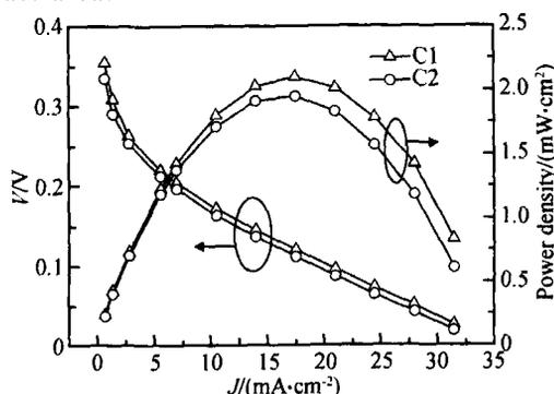
Fig. 6 Performance of the two types of air-breathing cathode designs. 2M methanol, 0.20mL/min, room temperature (25 °C)
