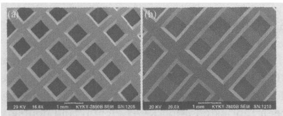
Fig. 2 SEM photos of C1 ,one type of the air-breathing cathode plate (a) Front side (in contact with the MEA) of C1 ;(b) Back side (facing the ambient) of C1
