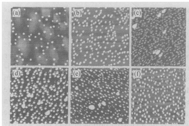
Fig.1 AFM images (a) ~ (f) of InAs QDs of samples 1A ~ 1F grown by MBE on GaAs (001) substrate ( $1\mu\text{m} \times 1\mu\text{m}$  area for all images)
