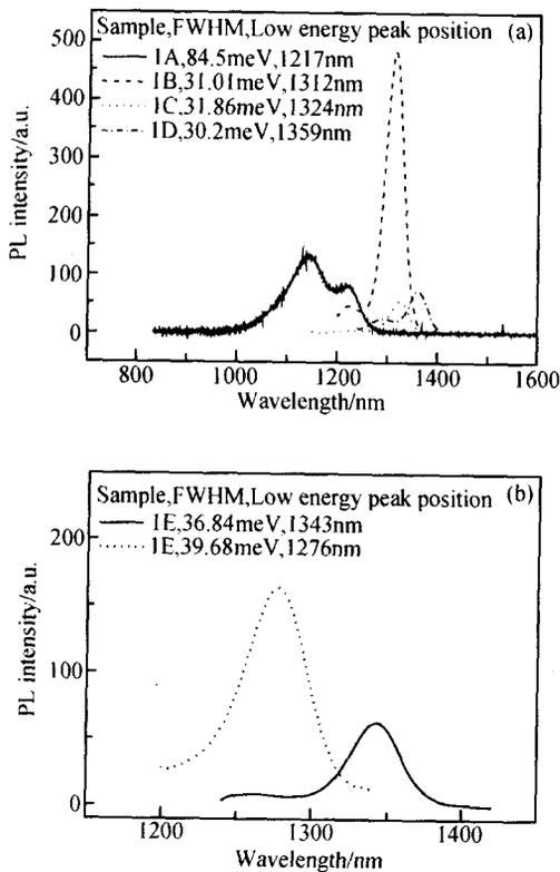
Fig. 2 PL spectra of samples 1A ,1B ,1C ,and 1D (a) , and 1E and 1F (b) at room temperature with an excitation power of 16mW
