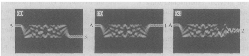
Fig. 2 Simulated switching states of the photonic switch when an input light is coupled into input waveguide A (a) Switched to output 3; (b) Switched to output 1; (c) Switched to output 2
