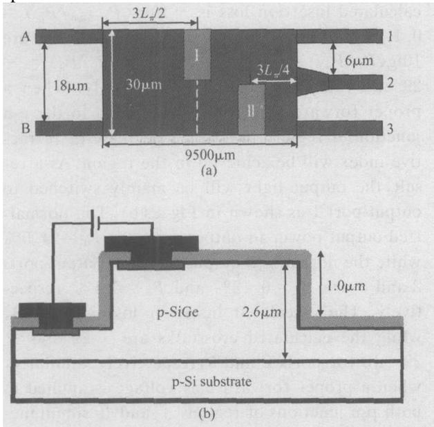
Fig. 1 Schematic structure of the proposed 2 ×3 photonic switch (a) Top view of the photonic switch; (b) Cross-section of the index-modulation regions
