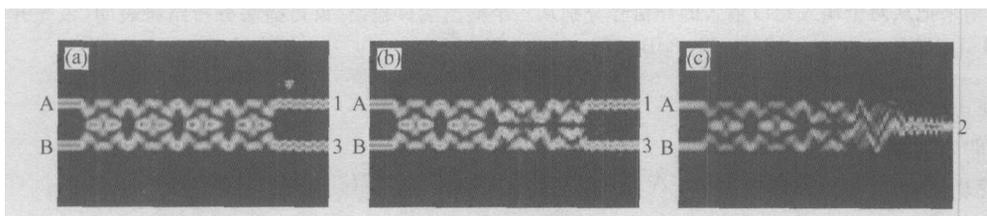
Fig. 4 Simulated switching states of the photonic switch when input lights are coupled into A and B simultaneously (a) Cross-state; (b) Bar-state; (c) Combined-state
