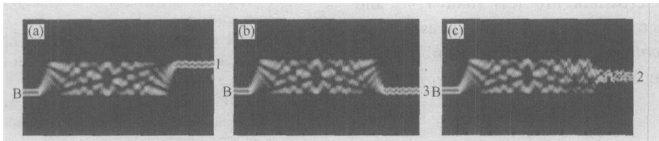
Fig. 3 Simulated switching states of the photonic switch when an input light is coupled into input waveguide B (a) Switched to output 1; (b) Switched to output 3; (c) Switched to output 2
