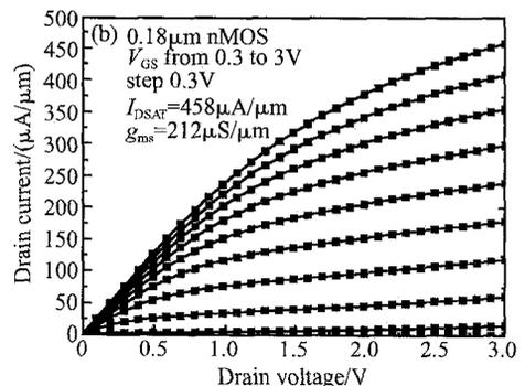
Fig. 3 DC characteristics of 0.18μm RF nMOSFET (a) Transfer characteristics; (b) Output characteristics
