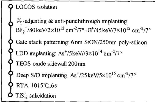
Fig. 1 Process flow for 0.18μm RF nMOSFET
