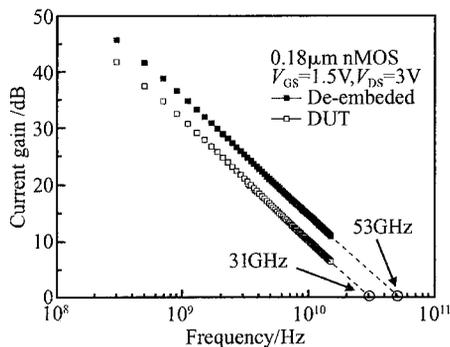
Fig. 4 Current gain versus frequency of 0.18 $\mu\text{m}$  nMOSFET
