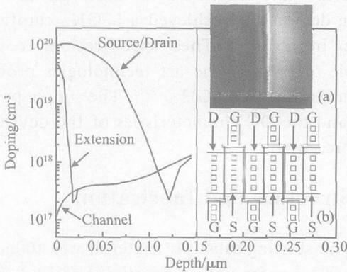
Fig. 2 Simulated doping profiles. Insets are SEM image of 0.18μm gate line (a) and multi-finger gate structure (b).
