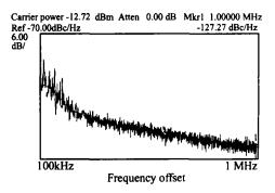
Fig. 7 Phase noise performance of VCO Carrier frequency is 1. 14 GHz
