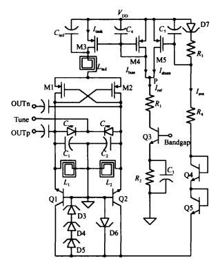
Fig. 2 Schematic of the VCO with AAC
