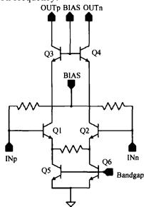
Fig. 6 Schematic of VCO buffer
