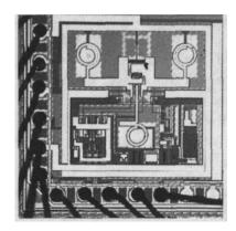
Fig. 10 Photomicrograph of the AAC VCO and buffer
