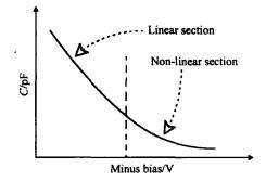
Fig. 4 Varactor capacitor versus tuning voltage
