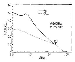
Fig. 6 RF characteristic :extrapolation to approximately 77 GHz of current gain cutoff frequency  $(f_T)$
