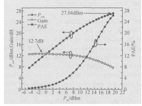
Fig. 7 Power performance of the 80  $\times 10 \mu m$  device (f = 8 G Hz; V\_{ds} = 10 V)
