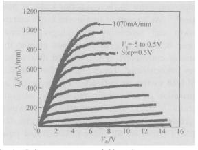
Fig. 5 Pulse measurement of 80  $\times 10\mu$ m power device s I-V curves
