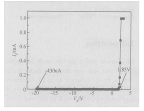
Fig. 4 Forward and reverse gate diode characteristics  $(W_g = 40 \mu m)$
