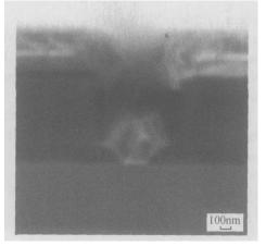
Fig. 2 SEM photo of 0. 25µm T-shaped gate
