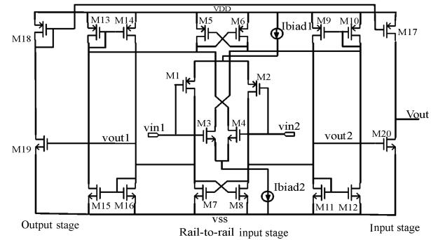
Fig.6. Rail-to-rail comparator with hysteresis function.
