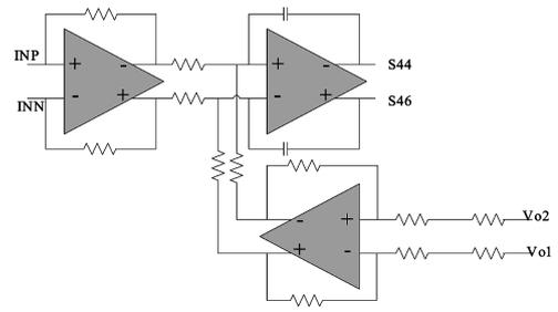
Fig.2. Diagram of preamplifier and feedback circuit.
