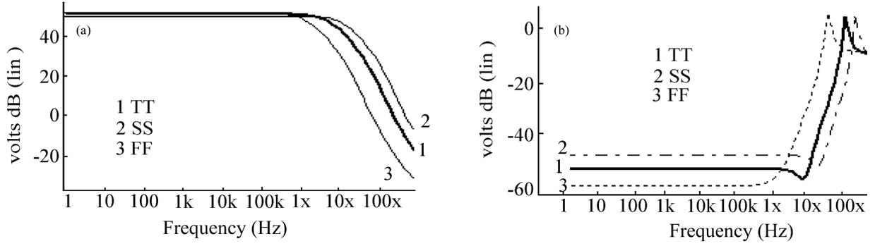
Fig.7. AC characteristics of PWM comparator: (a) DC gain; (b) PSRR.
