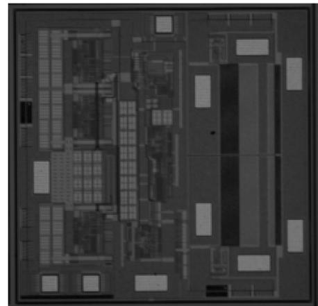
Fig.12. Micro-photo of the class-D amp.
