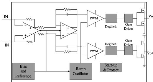
Fig.1. Diagram of class-D audio power amplifier.
