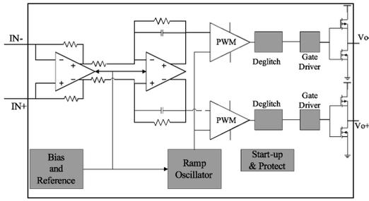
Fig.1. Diagram of class-D audio power amplifier.
