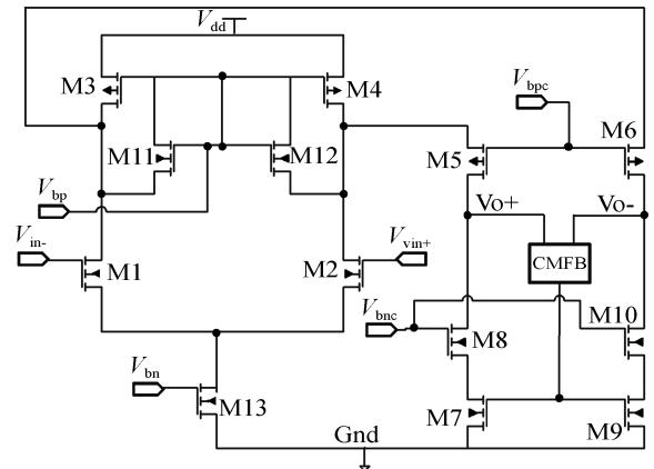
Fig.3. Full differential operational amplifier circuit.
