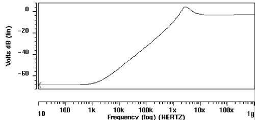
Fig.5. Power-supply rejection ratio characteristic of CMOS operational amplifier.
