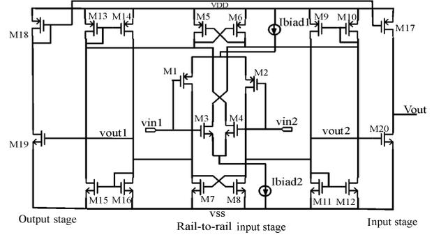
Fig.6. Rail-to-rail comparator with hysteresis function.
