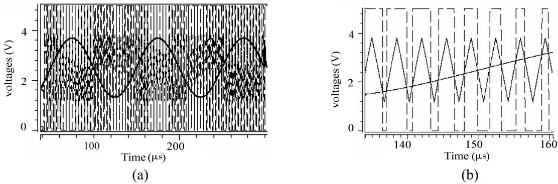
Fig.10. Output waves of PWM comparator: (a) Comparator output; (b) Amplified output waves.
