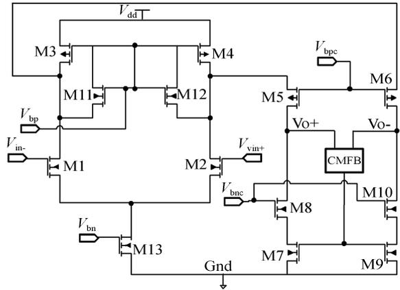
Fig.3. Full differential operational amplifier circuit.
