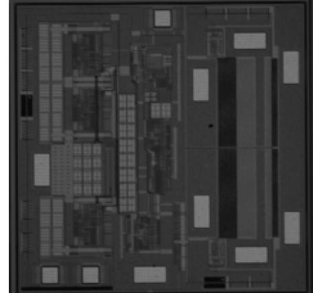
Fig.12. Micro-photo of the class-D amp.
