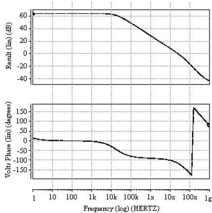
Fig.4. CMOS operational amplitude/phase-frequency characteristic.
