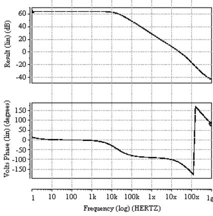
Fig.4. CMOS operational amplitude/phase-frequency characteristic.
