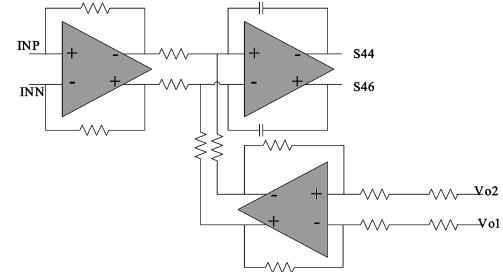
Fig.2. Diagram of preamplifier and feedback circuit.
