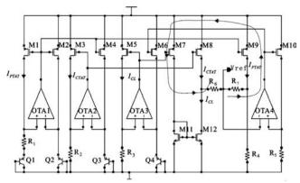
Fig. 2. Bandgap reference circuit.
