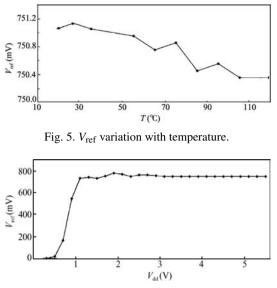
Fig. 6. V<sub>ref</sub> variation with supply voltage.
