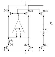
Fig. 1. Typical CMOS BGR.
