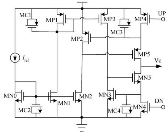
Fig. 7. Improved gain-boosting charge-pump.
