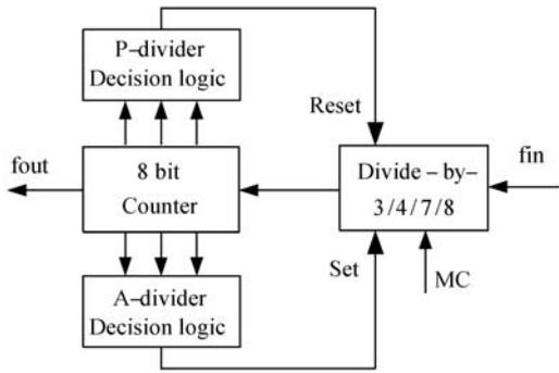
Fig. 5. Configuration of the multi-modulus divider.
