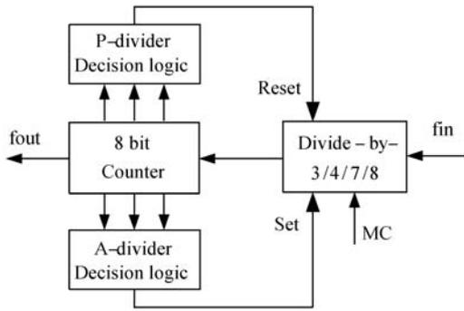
Fig. 5. Configuration of the multi-modulus divider.
