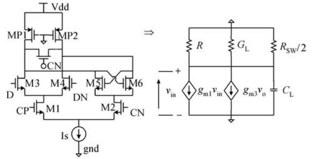
Fig. 4. Equivalent small signal model of the proposed latch.
