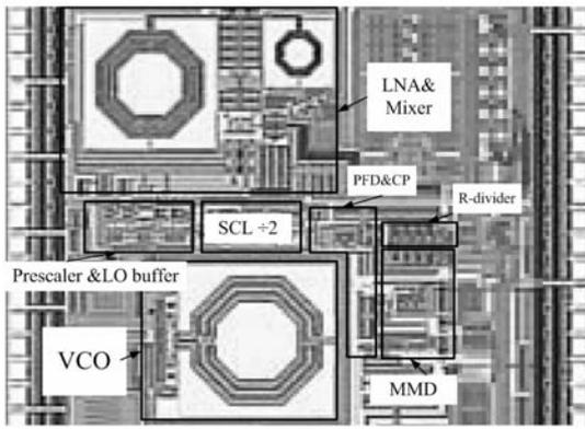
Fig. 9. Die photograph of the proposed synthesizer.
