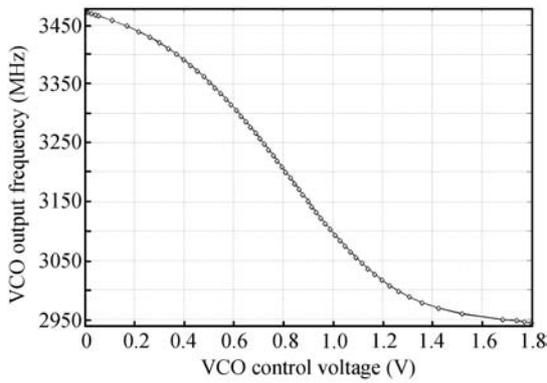
Fig. 10. Measured VCO tuning range.
