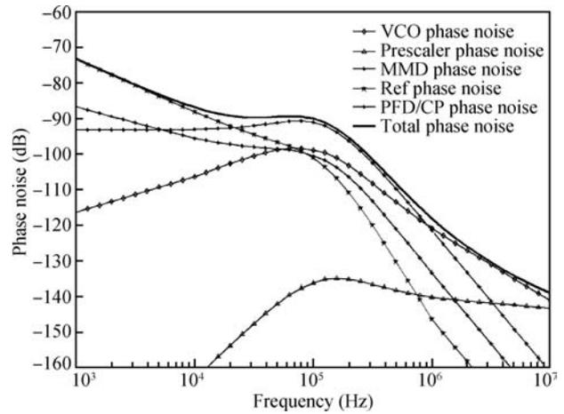
Fig. 8. Predicted total phase noise at the synthesizer output.
