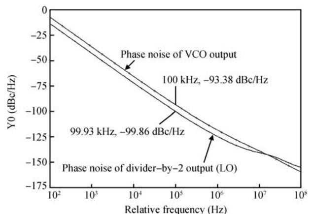
Fig. 1. Phase noise of the output of the prescaler and the VCO.
