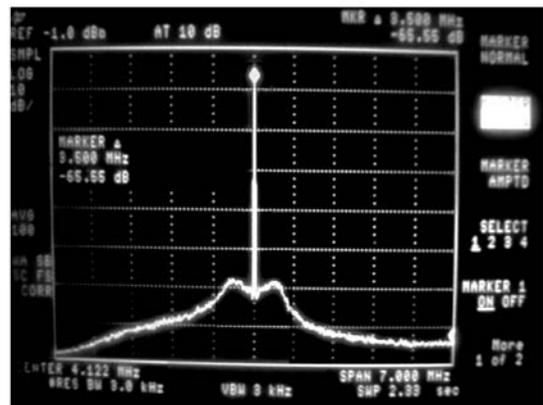
Fig. 14. IF signal with 7 MHz span.
