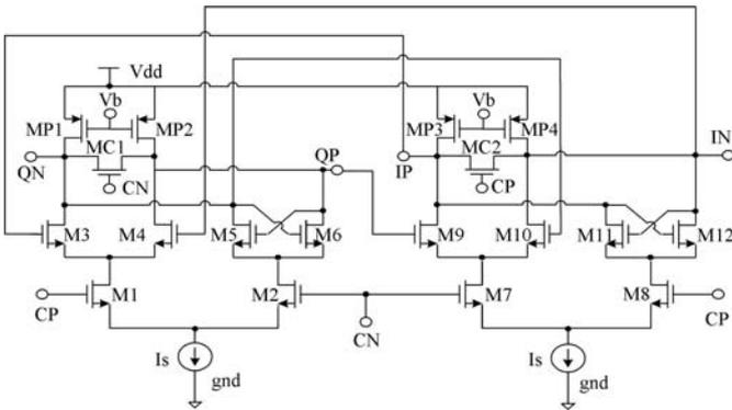
Fig. 3. Proposed prescaler based on a novel latch.
