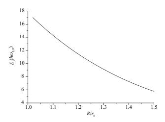
Fig. 3. Relational curves of the first internal excited state energy  $E_1$  with the transverse radius *R* of quantum rods for fixed  $l_p = 2$ ,  $l_v = 3$ , L = 5.5 and  $\alpha = 4$ .
