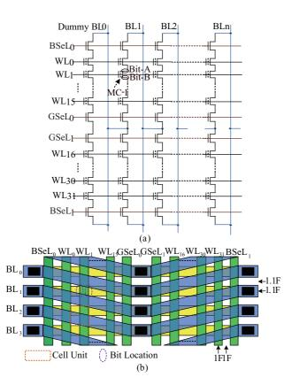
Fig. 4. (a) Schematic diagram of the proposed virtual-source NAND type array structure. (b) Top view layout of the proposed VS-NAND structure.
