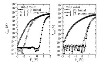
Fig. 7.  $I_{\text{drain}}/I_{\text{source}}-V_{\text{g}}$  curve of the NUC-CTM with different states of bit-A and bit-B.
