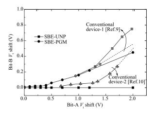
Fig. 8. SBE-UNP and SBE-PGM induced  $V_t$  shifts in the NUC-CTM and other mirror-bit storage devices<sup>[9, 10]</sup>.
