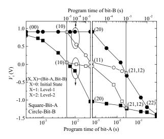
Fig. 9. 3-bit/cell storage characteristic of NUC-CTM and the program speed of each bit.
