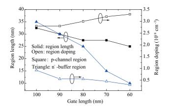
Fig. 2. Simulation results of scalability of NUC-CTM. The gate length can scale down below 60 nm by carefully controlling the length and doping of the p-channel region and the n<sup>-</sup>-type buffer region.
