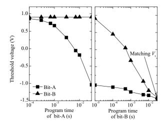
Fig. 6. Restrain on the interference between bit-A and bit-B during program operation.
