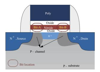
Fig. 1. Structure of a single NUC-CTM cell.
