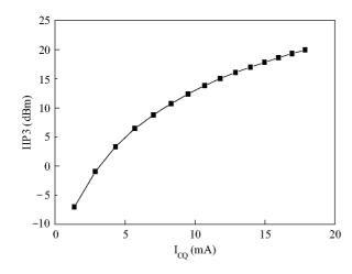
Fig. 5. Measurement curve of IIP3 versus  $I_{CQ}$ .
