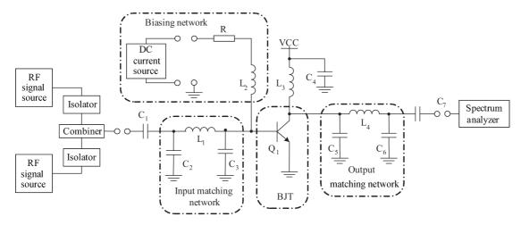
Fig. 4. Circuit used in two-tone test.
