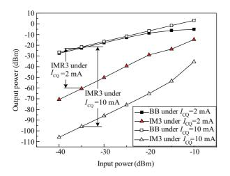
Fig. 7. Comparison of power level of output base-band signal and intermodulation product under different bias currents. BB means baseband signal, while IM3 means 3rd-order intermodulation.
