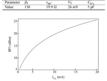
Fig. 3. Calculation curve of IIP3 versus  $I_{CO}$ .
