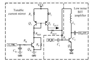
Fig. 6. Schematic of dynamic bias current LNA.
