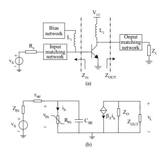
Fig. 1. (a) Typical CE BJT amplifier schematic and (b) its equivalent nonlinear circuit for a Volterra series calculation.
