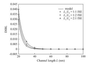
Fig. 5. Drain induced barrier lowing (DIBL) versus channel length L.
