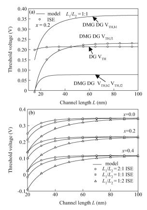
Fig. 4. Variation in threshold voltage along the channel for 100 nm DMG DG and DG MOSFETs. (a) Threshold voltage of DMG DG and DG MOSFETs. (b) Threshold voltage of DMG DG MOSFET changes with the gate length ratio and strain *X*.
