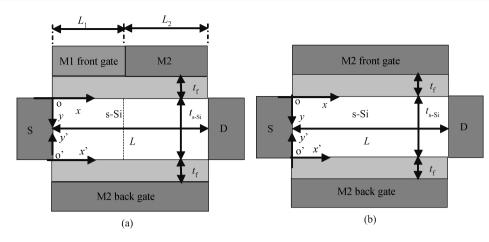
Fig. 1. Schematic structure of (a) a asymmetrical DMG DG strained-Si MOSFET and (b) a symmetrical DG strained-Si MOSFET.
