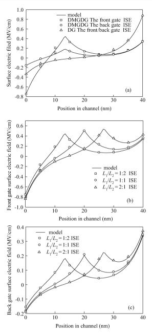
Fig. 3. Variation in the surface electric field within the channel for the 40 nm DMG DG and DG MOSFETs. (a) Surface electric field distribution of the front gate and the back gate surface of the DMG DG and DG MOSFETs. (b) Surface electric field distribution of the front gate of the DMG DG and DG MOSFETs. (c) Surface electric field distribution of the back gate of the DMG DG and DG MOSFETs.
