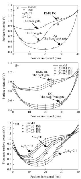
Fig. 2. Variation in the surface potential along the channel for the 40 nm DMG DG and DG strained-Si MOSFET. (a) Potential distribution of the front gate and back gate surface of the DMG DG and DG MOSFETs. (b) Potential distribution of the back gate surface of the DMG DG and DG MOSFETs. (c) Potential distribution of the front gate surface of the DMG DG MOSFETs.
