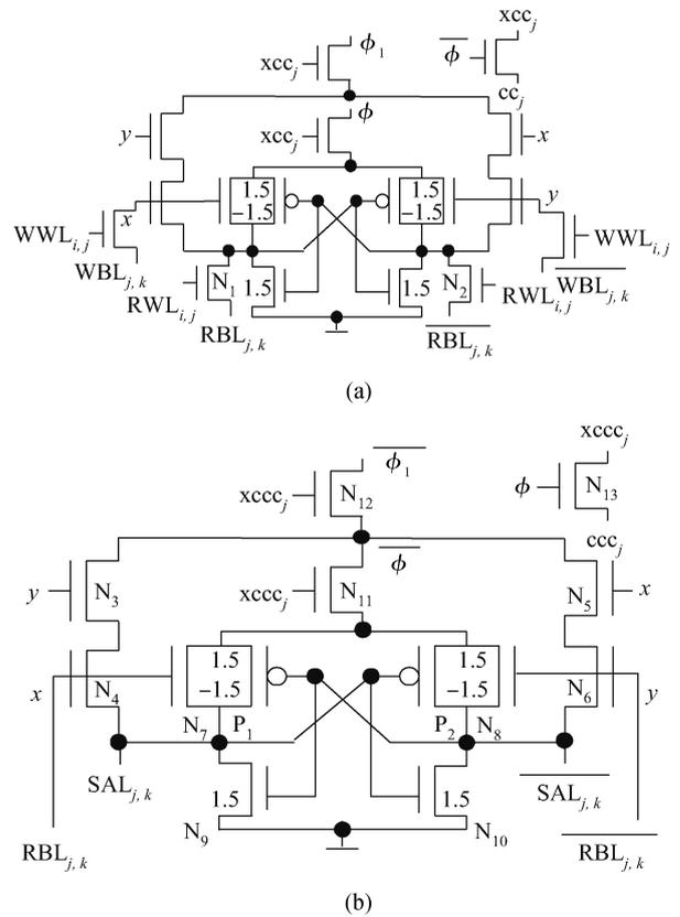
Fig. 5. (a) Storage cell. (b) Sense amplifier.
