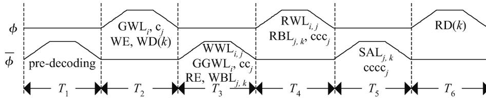
Fig. 6. Operation timing of ternary adiabatic SRAM.
