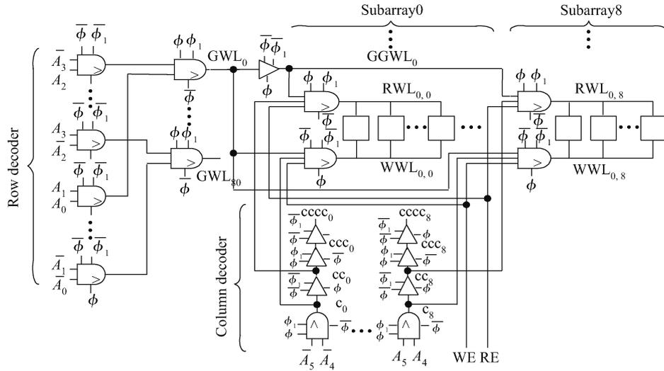
Fig. 3. Row/column address decoder.
