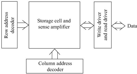
Fig. 2. Block diagram of ternary adiabatic SRAM.
