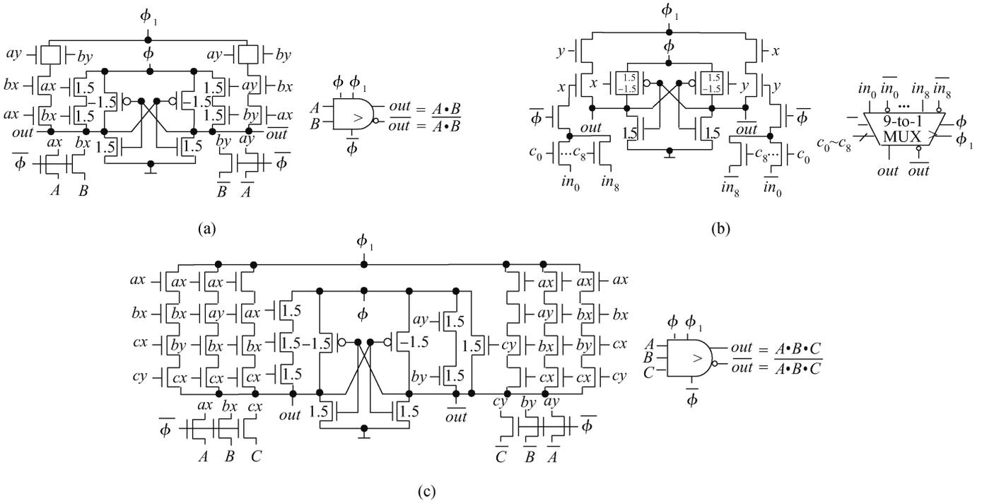
Fig. 1. DTCTGAL circuits. (a) Two-input AND gate. (b) 9 to 1 multiplexer. (c) Three-input AND gate.
