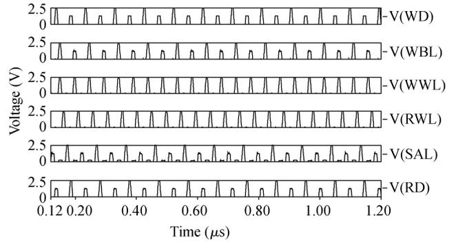
Fig. 7. Simulation waveforms of ternary adiabatic SRAM.
