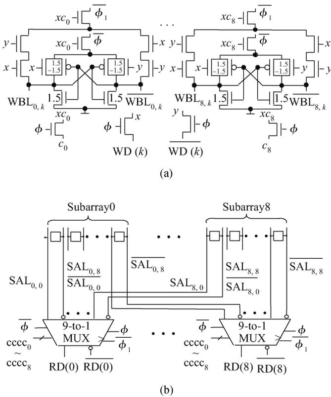
Fig. 4. (a) Write driver. (b) Read driver.
