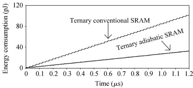
Fig. 8. Transient energy consumption comparison between ternary adiabatic SRAM and conventional SRAM.
