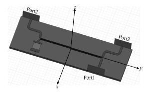
Fig. 1. Lange coupler's three-dimensional model of Ansoft HFSS.
