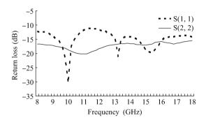
Fig. 12. The measured small-signal return loss of the amplifier.
