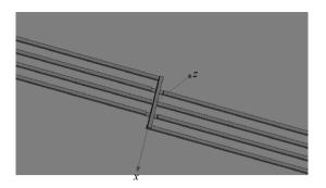
Fig. 2. Finger-to-finger structure of the Lange coupler.
