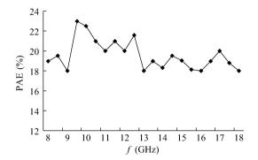
Fig. 9. Power-added efficiency ( $V_d = 8 \text{ V}, P_{in} = 25 \text{ dBm}$ ).
