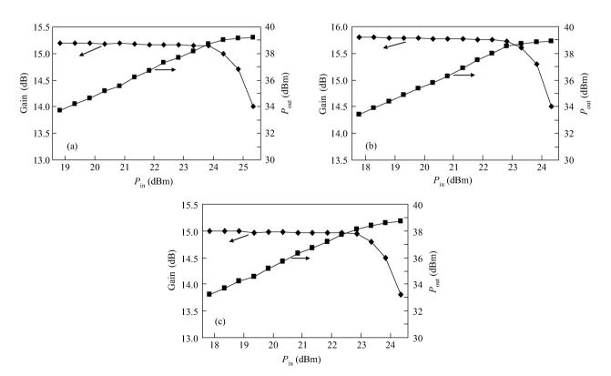
Fig. 10. Gain and power performance at (a) 8 GHz, (b)12 GHz, (c) 18 GHz.
