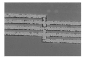
Fig. 3. Photograph of the finger-to-finger structure of the Lange coupler.
