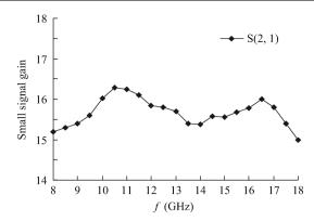
Fig. 11. The measured small signal gain ( $P_{in} = 18 \text{ dBm}$ ).
