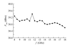
Fig. 8. Saturated output power ( $V_d = 8 \text{ V}, P_{in} = 25 \text{ dBm}$ ).
