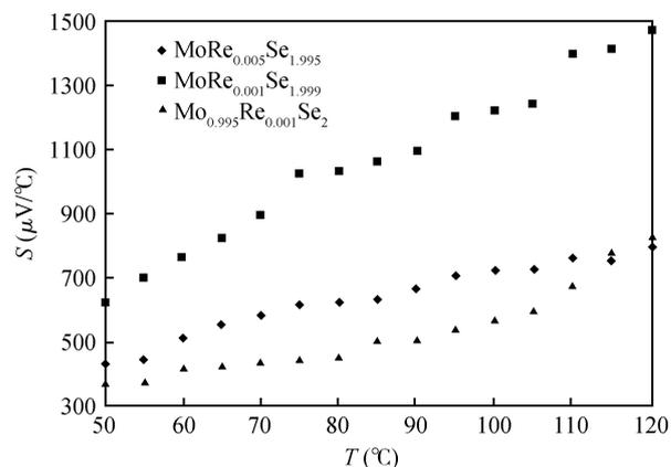
Fig. 4. Seeback coefficient ( $S$ ) ( $\mu\text{V}/^\circ\text{C}$ ) of Re-doped MoSe<sub>2</sub> single crystals.
