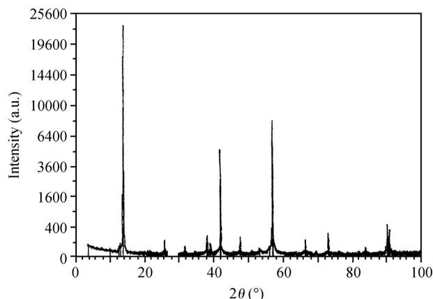
Fig. 2. X-ray diffractogram of MoRe<sub>0.001</sub>Se<sub>1.999</sub> single crystal.
