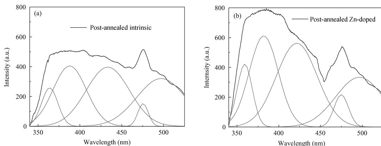
Fig. 5. Photoluminescence spectra of (a) post-annealed intrinsic  $\beta$ -Ga<sub>2</sub>O<sub>3</sub> films and (b) Zn-doped  $\beta$ -Ga<sub>2</sub>O<sub>3</sub> films.
