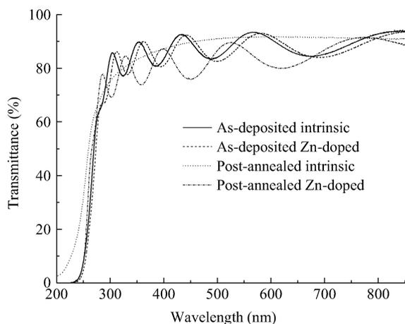
Fig. 2. Optical transmittance of as-deposited  $\beta$ -Ga<sub>2</sub>O<sub>3</sub> films and post-annealed  $\beta$ -Ga<sub>2</sub>O<sub>3</sub> films.
