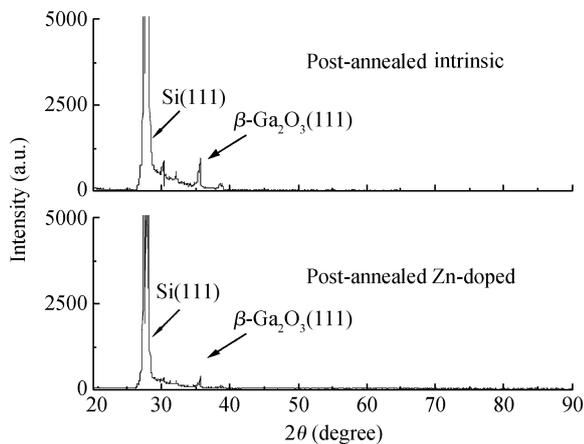
Fig. 1. XRD patterns of intrinsic  $\beta$ -Ga<sub>2</sub>O<sub>3</sub> films and Zn-doped  $\beta$ -Ga<sub>2</sub>O<sub>3</sub> films deposited on a Si substrate and post-annealed in vacuum at 800 °C for 2 h.
