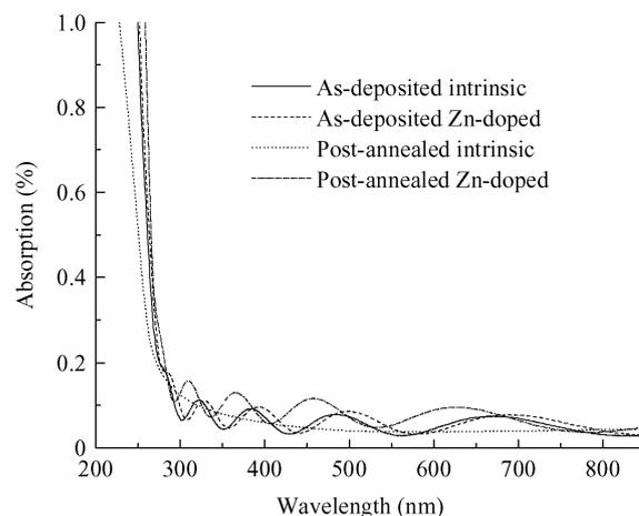
Fig. 3. Optical absorption of as-deposited  $\beta$ -Ga<sub>2</sub>O<sub>3</sub> films and post-annealed  $\beta$ -Ga<sub>2</sub>O<sub>3</sub> films.
