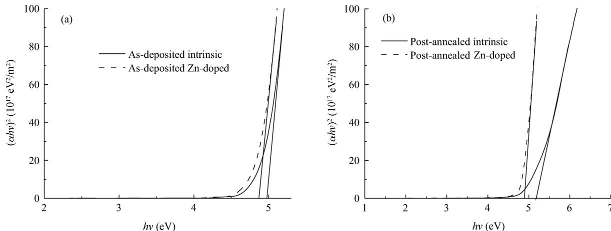
Fig. 4. (a) Optical band gap of as-deposited intrinsic  $\beta$ -Ga<sub>2</sub>O<sub>3</sub> films and Zn-doped  $\beta$ -Ga<sub>2</sub>O<sub>3</sub> films. (b) Optical band gap of post-annealed intrinsic  $\beta$ -Ga<sub>2</sub>O<sub>3</sub> films and Zn-doped  $\beta$ -Ga<sub>2</sub>O<sub>3</sub> films.
