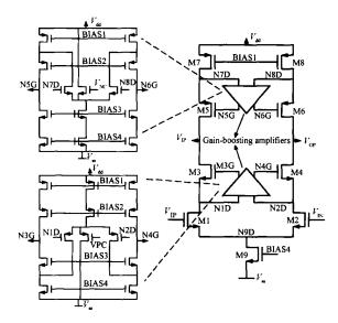
Fig. 4 Low-power high-bandwidth gain-boosting opamp
