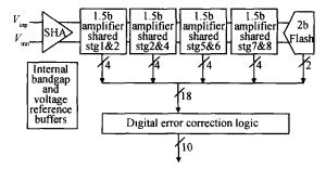
Fig. 1 Block diagram of the ADC
