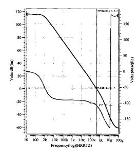
Fig. 5 Simulated gain and phase of the gain boosting opamp
