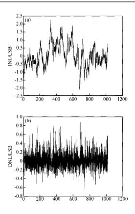
Fig. 9 Measured nonlinearity 40 Ms/s,  $f_{\text{in}} = 500 \text{ kHz}$
