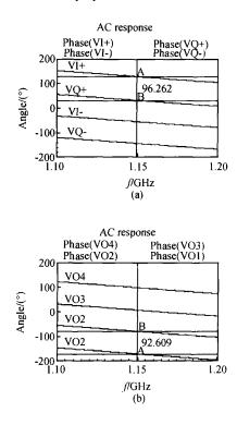
Fig. 8 Simulated phase error without (a) and with PMCC (b) with by Spectra RF
