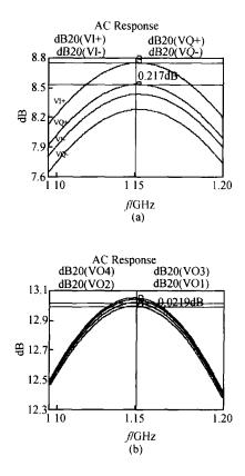
Fig. 7 Simulated amplitude difference without (a) and with PMCC (b) by Spectra RF
