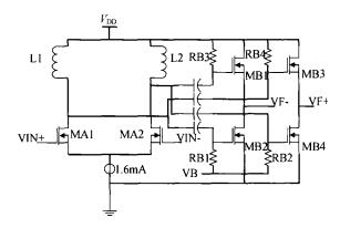
Fig. 2 Schematic of high frequency amplifier
