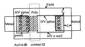
Fig. 6 Layout of HV-nMOS
