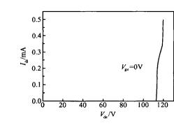
Fig. 4 Breakdown voltage of HV-nMOS devices
