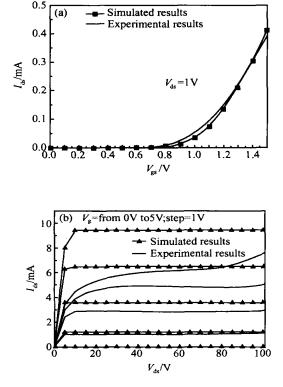
Fig. 3 Simulated results versus experimental results (a)  $I_{ds}$ - $V_{gs}$  characteristics; (b) Output characteristics
