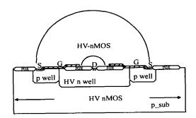
Fig. 8 Self-enclosed HV-nMOS
