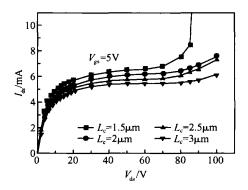
Fig. 5 Output characteristics of different channel
