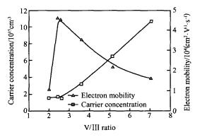
Fig. 1 Electron mobility and concentration of InP as functions of P/ In BEP ratio at 77 K
