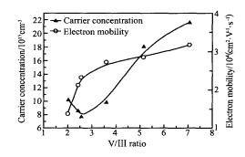
Fig. 2 Electron mobility and concentration of InP as functions of P/ In BEP ratio at 300 K
