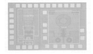
Fig. 6 Micrographic of frequency synthesizer
