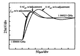
Fig. 8 Channel switching responses of control voltage for variation factor adjustment test, with 60 % extra current reduction
