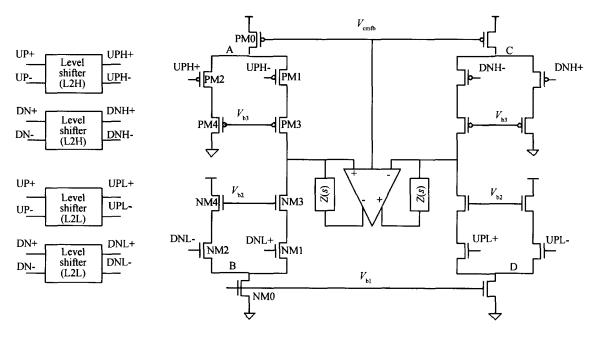
Fig. 3 Differential charge pump schematic
