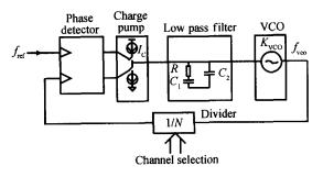
Fig. 1 Architecture of frequency synthesizer
