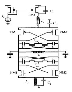
Fig. 5 Differential complementary cross-coupled-begative- $G_m$  VCO with cross-switched varactor
