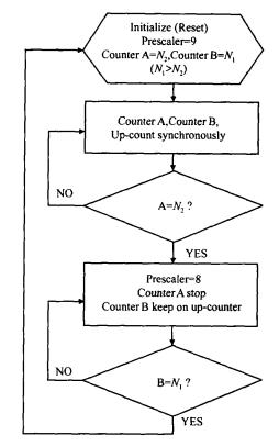
Fig. 5 Behavior flow diagram of down scalers
