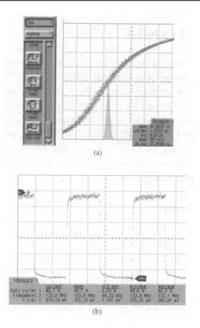
Fig. 4 Measured waveform of the high speed DMP (a) Measured jitter waveform; (b) Output of the DMP at divide-by-8
