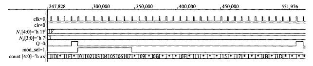
Fig. 6 Post-simulation waveforms of 9-bits programmable divider
