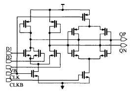
Fig. 3 D-latch architecture with 'OR 'logic input
