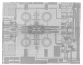
Fig. 6 Microphotograph of the frequency synthesizer
