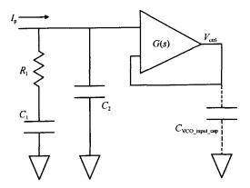
Fig. 3 Topology of a equivalent third order loop filter
