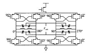
Fig. 1 Circuit diagram of QVCO
