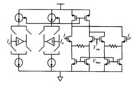
Fig. 2 Circuit diagram of differential charge pump
