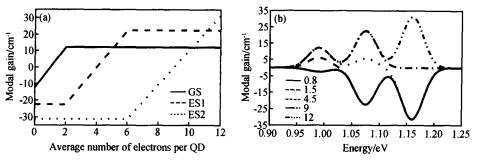
Fig. 2 (a) Norrequilibrium modal gain at center energy; (b) Norrequilibrium modal gain versus injection intensity
