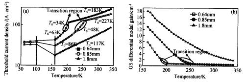
Fig. 5 (a)  $T_0$  and  $J_{th}$  for QDs lasers with different cavity lengths; (b) GS differential modal gain at threshold level versus temperature
