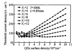
Fig. 7  $J_{\text{th}}$  versus  $n_{\text{QD}}$  as  $N_1$  increases from 2 to 12
