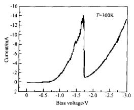
Fig. 2 FV curve of RTD with a 4µm ×4µm emitter PVCR = 13. 98 with  $I_p$  = - 0. 014309A,  $V_p$  = - 1. 68V,  $I_v$  = - 0. 0010236A,  $V_v$  = - 1. 707V
