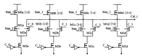
Fig. 5 Core structure of DAC \_ 2
