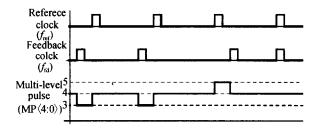
Fig. 3 Reference clock ,feedback clock ,and multi-level pulse MP 4 0
