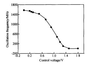
Fig. 7 VCO frequency versus the control voltage Ctr \_ v
