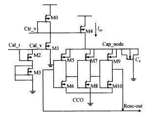
Fig. 6 Core structure of VCO
