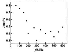
Fig. 10 Measured frequency peak-to-peak jitter versus DPLL output frequency
