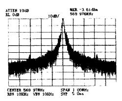
Fig. 11 Output spectrum of the DPLL
