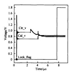
Fig. 9 Simulated Cal \_ v ,Ctr \_ v ,and lock flag
