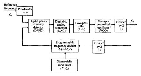
Fig. 1 DPLL functional block diagram
