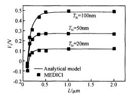
Fig. 4 Threshold voltage versus gate length for different silicon film thicknesses The devices parameters are:  $T_{\text{fox}} = 10$  nm ,  $T_{\text{box}} = 320$  nm ,  $N_{\text{ch}} = 1.2 \times 10^{17}$  cm<sup>-3</sup> ,  $V_{\text{ds}} = 0.05$  V.
