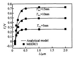
Fig. 3 Threshold voltage versus gate length for different gate oxide thicknesses The device parameters are:  $T_{\rm Si} = 100$  nm,  $T_{\rm box} = 320$  nm,  $N_{\rm ch} = 1.2 \times 10^{17}$  cm<sup>-3</sup>,  $V_{\rm ds} = 0.05$  V.
