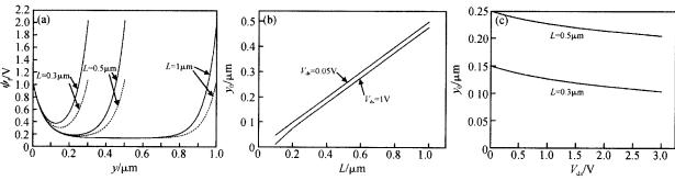
Fig. 2 (a) Calculated front surface potential distribution The device parameters are:  $T_{\text{fox}} = 10$  nm,  $T_{\text{Si}} = 100$  nm,  $T_{\text{box}} = 10$ 320nm,  $N_{ch} = 1.2 \times 10^{17} \text{ cm}^{-3}$ . The substrate bias is 0V. The dashed lines show the data for  $V_{ds} = 0.05V$ , and the solid lines for  $V_{ds} = 1V$ ; (b) Calculated location of potential minimum as a function of channel length; (c) Calculated location of potential minimum as a function of drain voltage
