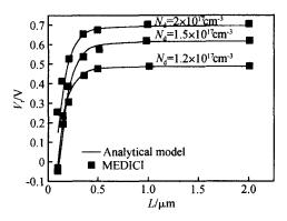
Fig. 5 Threshold voltage versus gate length for different channel doping concentrations The devices parameters are :  $T_{\text{fox}} = 10$  nm ,  $T_{\text{box}} = 320$  nm ,  $T_{\text{Si}} = 100$  nm ,  $V_{\text{ds}} = 0.05$  V.
