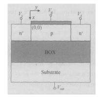
Fig. 1 Cross-section of an n-channel SOI MOSFET
