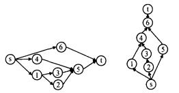
Horizontal constraint graph  $G_h$  Vertical constraint graph  $G_v$ Fig. 6 Adjacency graphs of packing of floorplanning on CBL
