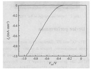
Fig. 5 Breakdown characteristics of gate-drain
