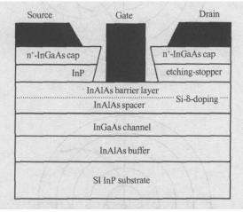
Fig. 1 Schematic cross-section of InP HEMT
