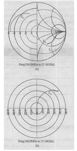
Fig. 6 S-parameters of InP HEMT (a)  $S_{11}$ ,  $S_{21}$ , and  $S_{22}$ ; (b)  $S_{12}$
