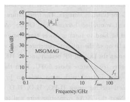
Fig. 7 Current gain and maximum available/ stable power gain
