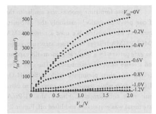
Fig. 3 *FV* characteristics of InP HEMT
