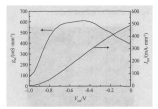
Fig. 4 IDS and gm versus V GS of InP HEMT
