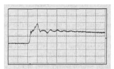
Fig. 3 Waveform of non-linear mode X:50 ns/ div, Y: 500 mV/ div
