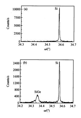
Fig. 2 X-ray diffraction of SiGe grown at 300 (a) and 450 (b)
