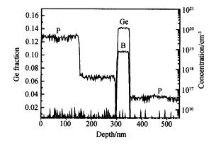
Fig. 3 SIMS profile of  $n \cdot Si$ /  $i - Si_{0..86}$  Ge<sub>0..14</sub>/  $p^+ - Si_{0..86}$ -Ge<sub>0..14</sub>/  $i - Si_{0..86}$  Ge<sub>0..14</sub>/ n - Si
