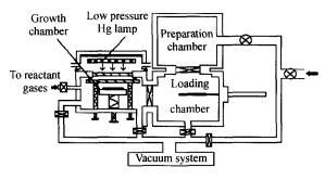
Fig. 1 Schematic of UV/UHV/CVD system
