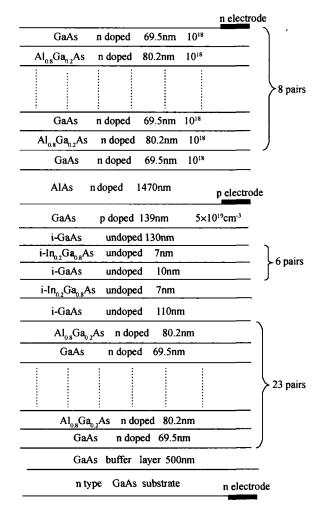
Fig. 1 Schematic diagram of epitaxial structure of the MOEMS tunable RCE photodetector
