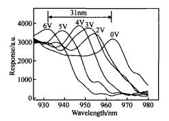
Fig. 5 Measured response spectra of the device under different tuning voltage The photodetector is biased by 3V DC.
