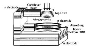
Fig. 2 Schematic structure of the MOEMS tunable RCE photodetector
