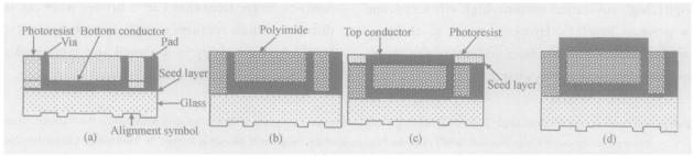
Fig. 2 Fabrication process for a complete inductor (a) Fabrication of alignment symbol ,electroplating bottom conductor ,via ,and pad; (b) Spinning and curing polyinmide ,and polishing polyimide until the vias were exposed; (c) Electroplating of top conductor; (d) Removal of seed layer
