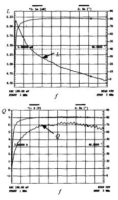
Fig. 4 Measured inductor parameter as a function of frequency (a) Inductance versus frequency; (b) Q factor versus frequency
