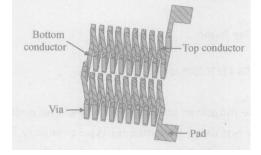
Fig. 1 Schematic diagram of a solenoid-type inductor
