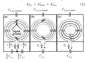
Fig. 1 Planar monolithic inductors with the same track width ,space ,inner ,and outer radius (a) Differentialdriven symmetric configuration (DSPI); (b) Single-ended-driven symmetric configuration (SSPI); (c) Singleended spiral configuration (SEPI) 1,2,3,4,5, and 6 are current flow direction in inductor, i. e. AC signal voltage profile or half-turns serial number; Capacitances are the equivalently parasitical capacitance of the monolithic inductor.
