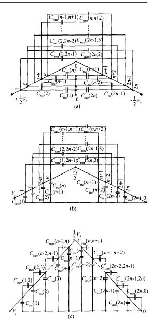
Fig. 2 Voltage profile and distributed capacitance model of the r turn planar inductor (a) DSPI; (b) SSPI; (c) SEPI
