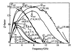
Fig. 6 Q and  $f_{SR}$  of two differential inductors with low  $C_{m_{m}}$   $L_3$  is the inductor in Fig. 5 (b) and  $L_5$  is the inductor in Fig. 5 (a) ; $L_4$  and  $L_6$  are the conventionally differential inductor with the same width and turns as  $L_3$  and  $L_5$ , respectively.
