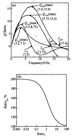
Fig. 4 (a) Q factor as a function of fregnency; (b) Ratio<sub>f SR</sub> as a function of Ratio<sub>C</sub> =  $C_{\text{m-n}}/C_{\text{m-s-diff}}$
