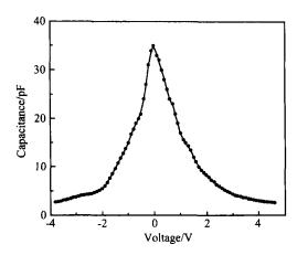
Fig. 4 C-V characteristics of Au/ n-ZnO SBD
