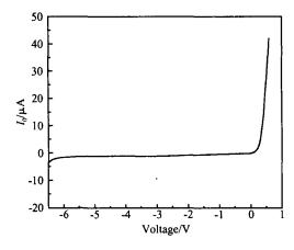
Fig. 5 FV characteristics of n-ZnO/p-Si
