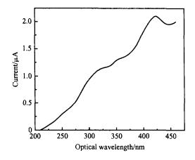
Fig. 6 Photo-current response at optical wavelengths
