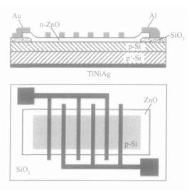
Fig. 1 Structure of the SHBT
