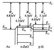
Fig. 2 Energy band of Au/ n-ZnO/ p-Si structure
