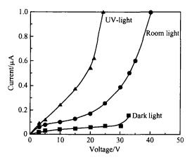
Fig. 3 FV characteristics of Au/ m ZnO SBD
