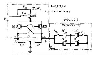
Fig. 2 Full schematic of the proposed VCO
