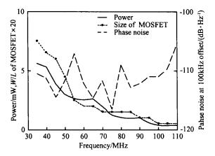
Fig. 5 Test results of phase noise at a 100k Hz offset, size of cross-coupled MOSFET in "on " mode, and core bias current
