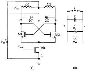
Fig. 1 CMOS LC VCO and its simplified circuit
