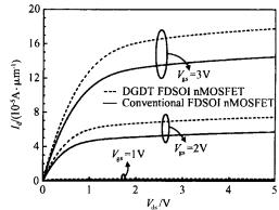
Fig. 7 Simulated output characteristics of the DG-DT and conventional FDSOI nMOSFET
