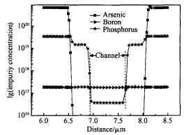
Fig. 3 Impurity concentrations along the channel region after process simulation
