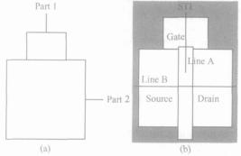
Fig. 1 (a) Layout of the active island composed of Part 1 and Part 2 Part 1 and the BOX layer below it will be partially etched off for the connection between the front-gate polysilicon and back-gate n-well; (b) Layout of the nMOSFET
