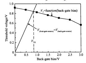
Fig. 6 Threshold voltage of FDSOI nMOSFET as a function of the back-gate-source forward bias  $V_{\rm T} (V_{\rm back-gate-source} = 0V) = 0.92V$ , but  $V_{\rm T} (V_{\rm back-gate-source} = 3V) = 0.56V$   $V_{\rm TH}$  represents the point where the gate bias of the DGDT FDSOI nMOSFET and the threshold voltage become identical.
