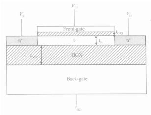
Fig. 5 Cross section of the four-terminal thin film FD-SOI nMOSFET
