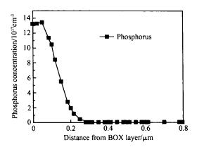
Fig. 4 Phosphorus concentration distribution beneath the BOX layer after process simulation
