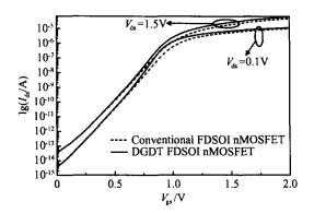
Fig. 8 Simulated  $I_{ds}$ - $V_{gs}$  characteristics of the conventional FDSOI and DGDT FDSOI nMOSFETs biasing at 0. 1 and 1. 5V
