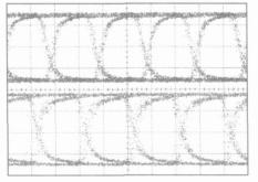
Fig. 15 Output eye diagrams of two adjacent front-end amplifiers
