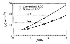
Fig. 7 Comparison of optimized RGC and conventional RGC in noise performance
