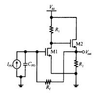
Fig. 3 Circuit diagram of the TIA
