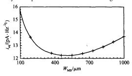
Fig. 6 Equivalent input noise current spectral density as a function of the gate width  $W_{\text{MB}}$
