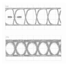
Fig. 14 (a) Output eye diagram with  $2mV_{pp}$  at 2. 5 Gb/s; (b) Output eye diagram with 0.  $8mV_{pp}$  at 2. 5 Gb/s
