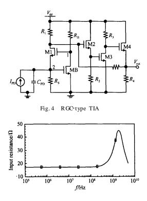
Fig. 5 Input resistance of RGC-type TIA
