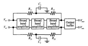
Fig. 9 Limiting amplifier structure
