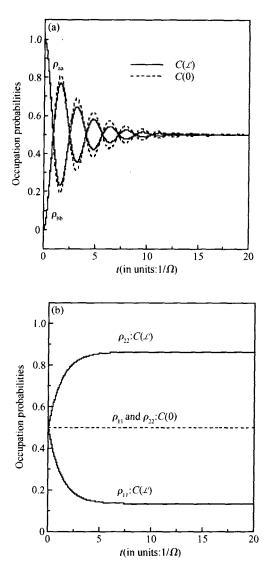
Fig. 2 Measurement induced qubit relaxation in the individual dot-state representation (a) and the eigenstate representation (b) The results in the presence and the absence of the detailed balance are symbolized by " C(L) " and " C(0) ", respectively.
