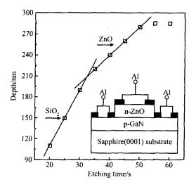
Fig. 1 Etching depth of  $SiO_2/ZnO$  as a function of etching time at room temperature Inset shows the diagram of n-ZnO/p-GaN heterojunction L ED device.
