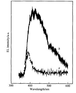
Fig. 3 Room temperature EL spectra of n-ZnO/p-GaN under forward-bias (a) and reverse-bias (b) voltages
