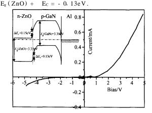
Fig. 2 Current-voltage relationship and energy-band diagram of an n-ZnO/p-GaN heterojunction device
