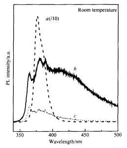
Fig. 4 Room temperature PL spectra of as-grown ZnO (curve a), GaN prior to ZnO growth (curve c), and also GaN sample (curve b) which has undergone ZnO growth and then been removed
