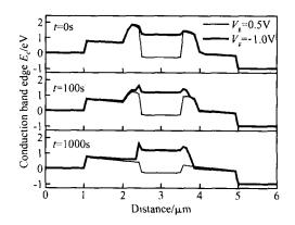
Fig. 7 Surface conduction band edge at different times for  $V_{\rm g}=0.\,5V$  and  $V_{\rm g}=$  -  $1.\,0V$
