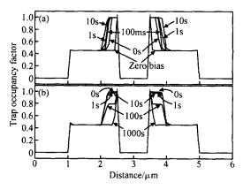
Fig. 5 Change of the trap occupancy factor  $F_n$  with time at the surface in the stress (a) and in the slow transient(b) The time reference is the moment immediately after the respective rise edge, and zero bias means the stable state.
