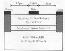
Fig. 1 Device structure The gray regions are taken to be GaN in the simulation.
