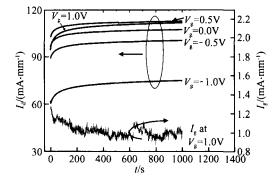
Fig. 2 Measured drain current transients at  $V_d = 1V$ under different  $V_g$  The gate current at  $V_g = 1V$  is also shown.
