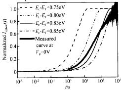
Fig. 4 Simulated  $I_{d,slow}$  (t) waveforms at different trap energy levels
