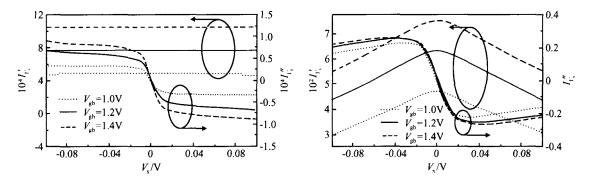
Fig. 4 Symmetry tests of drain current and its high-order derivatives in BSIM5 for 20 and 0.1µm MOSFET devices
