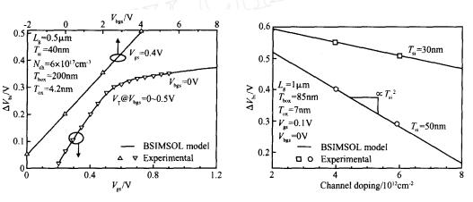
Fig. 11 Dependence of  $V_{bi}$  on front gate voltage and back gate voltage for the given structure and process parameters and on the channel doping for the given gate biases
