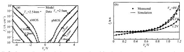
Fig.7 Gate tunneling current density versus gate voltage (a) and total gate tunneling current versus the source-drain voltage (b)
