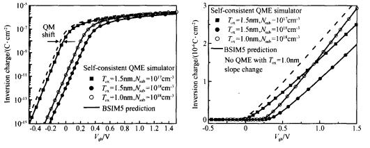
Fig. 1 Inversion charge comparison between the self-consistent simulation and BSIM5 prediction in the sub-threshold region and strong inversion region for different  $T_{ox}$  and dopings
