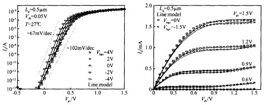
Fig. 13 Model verification of the PD-SOI and FD-SOI transition in BSIMSOI
