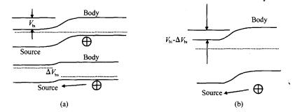
Fig. 10 Comparison of the energy bands of the PD-SOI (a) and FD-SOI (b) and the similarity of both via an effective body-source potential lowering  $V_{\rm bi}$
