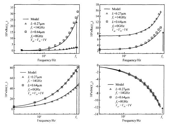
Fig. 6 Comparison of Y parameters of the two-port network MOS transistor between the BSIM4 prediction and the experimental measurements for different device channel lengths
