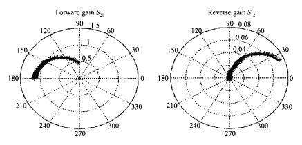
Fig. 14 Comparison of the S parameters between the measured and the BSIMSO13.2 prediction for a short channel MOS transistor for the frequency range  $100 \text{ MHz} \sim 20 \text{ GHz}$
