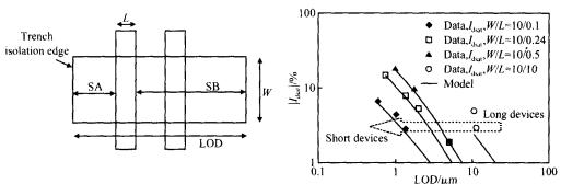
Fig. 9 Stress model parameters SA,SB and LOD layout dependence and comparison of the saturation drain current variation between the BSIM4 model and the measured data
