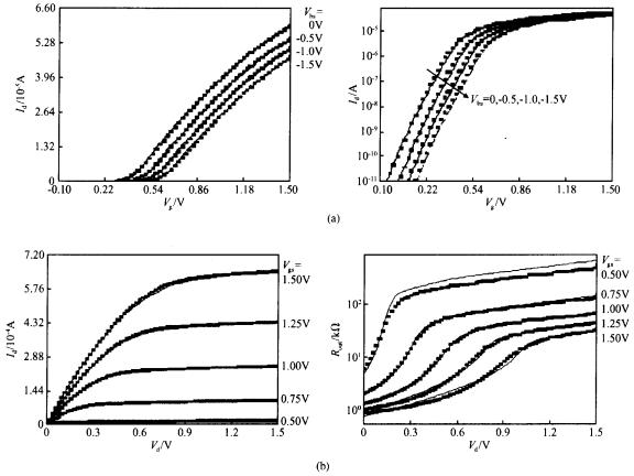
Fig. 2 (a) Comparison of  $I_{ds}$  versus  $V_{gs}$  between experimental data and BSIM5 fitting for 1µm MOSFET device; (b) Comparison of  $I_{ds}$  versus  $V_{ds}$  and  $R_{out}$  between experimental data and BSIM5 fitting for 1µm MOSFET device
