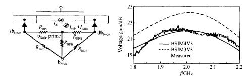
Fig. 5 BSIM4 substrate resistance network and RF function confinement from a prototype LNA was fabricated in 0.6µm CMOS
