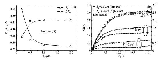
Fig. 12 Threshold voltage and  $V_{bi}$  variation with the decrease of the channel length (a) and comparison between BSIMSOI and the measured data for different device channel lengths (b)
