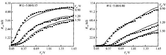
Fig. 8 Comparison of the output resistance between the BSIM4 and the measured values for different channel lengths and gate voltages
