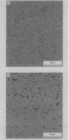
Fig. 4 Cross-sectional optical micrographs of the samples subjected to Ni annealed in groups A and B (a) MDZ annealing (RTP 1250 for 50s + 750 for 4h + 1050 for 16h) + Ni contamination by RTP (1000 for 50s); (b) Ni contamination by RTP (1000 for 50s) + MDZ annealing (RTP 1250 for 50s + 750 for 4h + 1050 for 16h)
