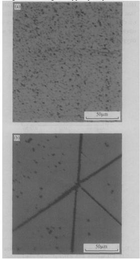
Fig. 3 Cross sectional optical micrographs of the samples subjected to Cu annealed in groups A and B (a) MDZ annealing (RTP 1250 for 50s + 750 for 4h + 1050 for 16h) + Cu contamination by RTP (1000 for 50s); (b) Cu contamination by RTP (1000 for 50s) + MDZ annealing (RTP 1250 for 50s + 750 for 4h + 1050 for 16h)
