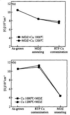
Fig. 1 Variation of interstitial oxygen concentration ([O<sub>i</sub>]) in samples with different copper contaminated sequences during IG annealing (a) MDZ annealing (RTP 1250 for 50s + 750 for 4h + 1050 for 16h) + Cu contamination by RTP (1000 / 1200 for 50s); (b) Cu contamination by RTP (1000 / 1200 for 50s) + MDZ annealing (RTP 1250 for 50s + 750 for 4h + 1050 for 16h)
