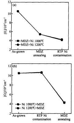
Variation of interstitial oxygen concentration Fig. 2  $([O_i])$  in samples with different nickel contaminated sequences during IG annealing (a) MDZ annealing (RTP 1250 for 50s + 750 for 4h + 1050 for 16h) + Ni contamination by RTP (1000 / 1200 for 50s); (b) Ni contamination by RTP (1000 / 1200 for 50s) + MDZ annealing (RTP 1250 for 50s + 750for 4h +1050for 16h)
