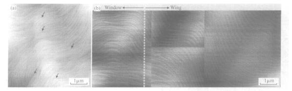
Fig. 3 (a) An AFM image of typical GaN film showing step terminations that are due to the intersection of either a pure screw or mixed threading dislocation with the film surface; (b) Montages of AFM images of successive  $4\mu m \times 4\mu m$  scans from window to wing, where dark arrows are shown as a guide to the eye to point out the step terminations
