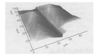
Fig. 5 50µm ×50µm AFM scan of ELOG GaN
