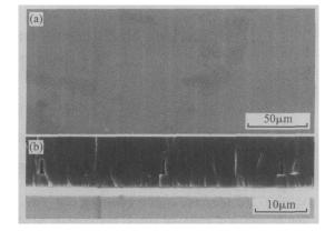
Fig. 1 Plane view (a) and cross-sectional view (b) of SEM images for coalesced ELOG GaN samples One of the merging front related contrast lines is highlighted by a vertical arrow.
